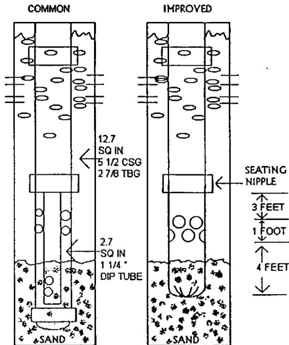
Fig. 1 Natural Gas Separators
