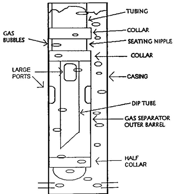
Fig. 5 Collar-Size Gas Separator in Casing
