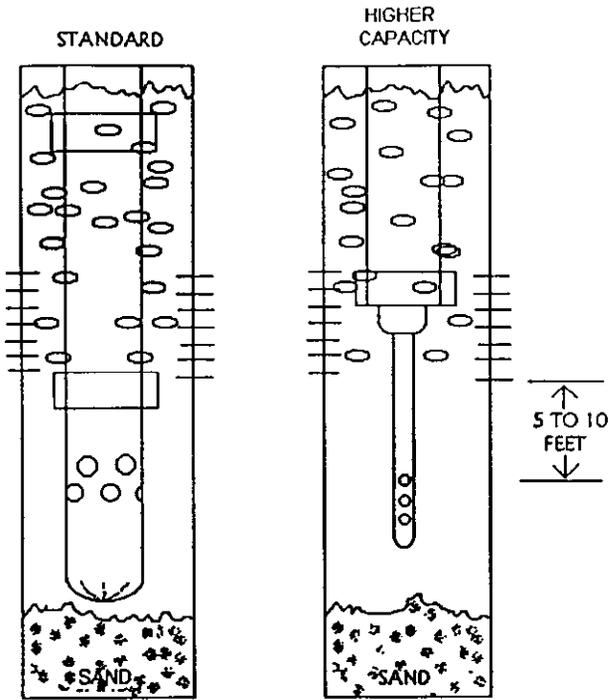
Fig. 2 Higher Capacity Natural Gas separator
