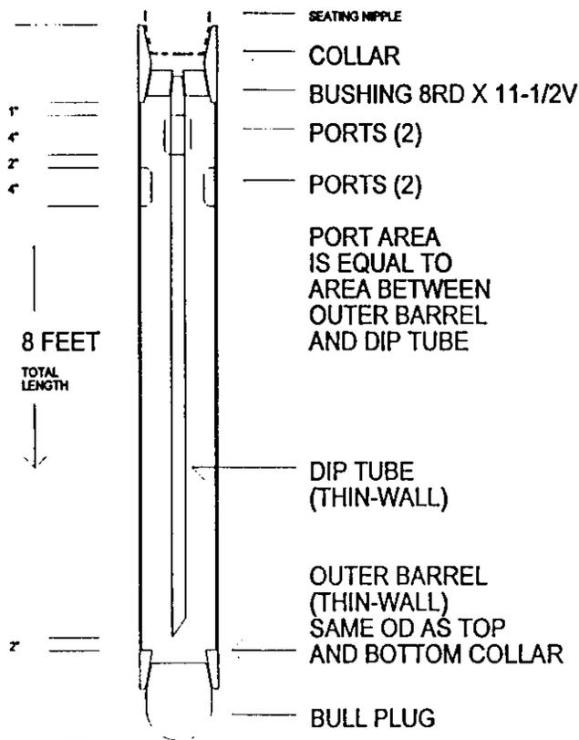
Fig. 4 COLLAR-SIZE GAS SEPARATOR DETAIL
