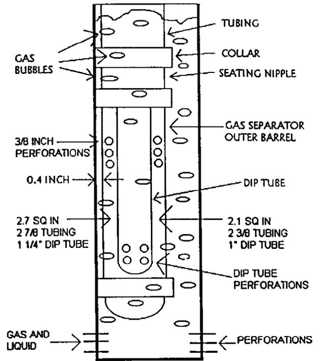
Fig. 3 Conventional Separator Above Formation
