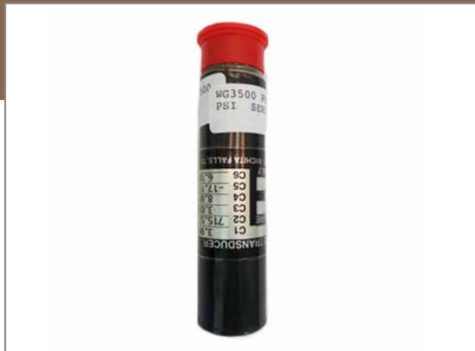
The pressure transducer also houses a thermistor that measures transducer temperature. All pressure measurements are temperature compensated. The pressure transducer is calibrated over a range of -40°F to 140°F. The temperature corrections are automatically applied by software.
